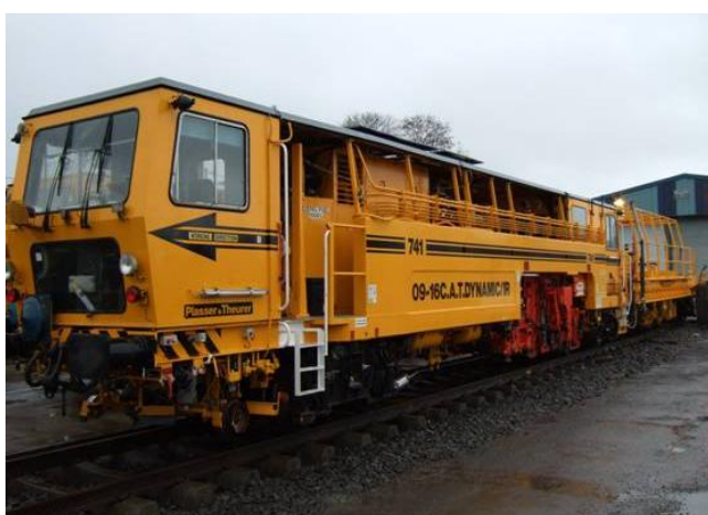
3.4-1 Plasser 09-16 continuous action tamper
