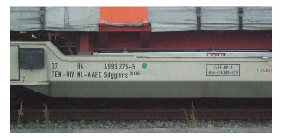
Note: Based on TSI 2008/107/EC the "TEN" marking generally required for freight wagons is not permitted to be put on wagons which are not of 1435mm gauge. Further the RIV marking is limited to Wagons which fully comply with all applicable RIV requirements.
