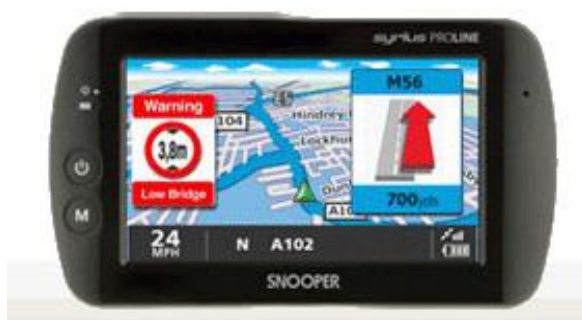
Figure 12: Sirius Proline with Truckmate Low bridge software
