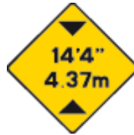
Figure 9: Reduced Headroom warning signage
