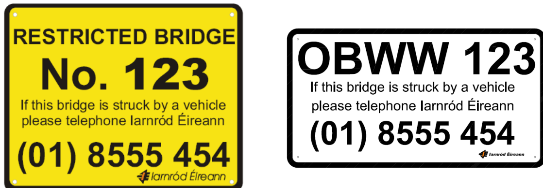
Figure 11: Height Restricted bridge (left) & over-bridge identification plates
