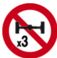
Figure 15: No entry to goods vehicles (by reference to number of axles)
